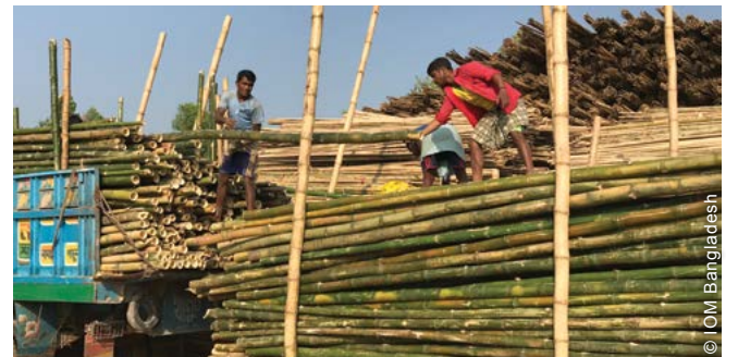
The procurement and logistics for the bamboo required for 100,000 kits needed a large dedicated team and the application of expedited procedures. Because of time constraints, bamboo was untreated and often harvested hurriedly.
