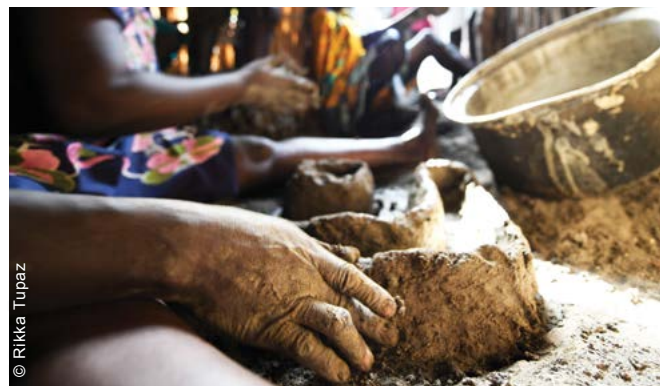
Stoves were made of local materials and according to traditional cooking practices. Women participated in the design of the stoves and were trained on how to construct them.
