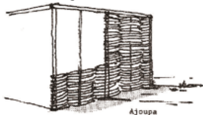
Kay Ajoupa (wattle or reed houses). Wood pole frame with woven cane or sticks as walling. Lived in by the poorest Haitians.
