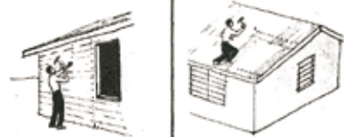
Hurricane preparedness: blocking gaps in the eaves and under shelters, securing walling and roofing sheets
