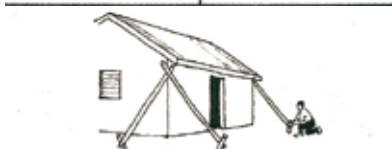
Hurricane preparedness: shuttering windows, building protective screens in front of openings and bracing corners of buildings
