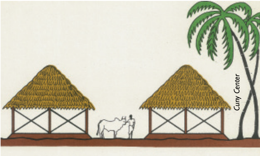
Shelter design elevation showing cross-bracing
