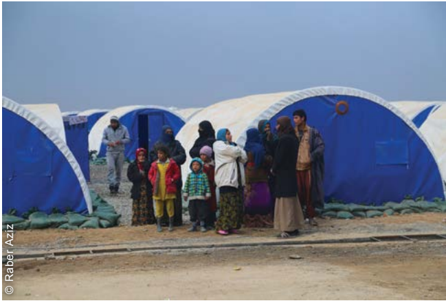
Using a rapid settlement approach, families were accommodated before all facilities and infrastructure were installed. Gravel was added in the shelter areas and roads excavated 20cm lower than the blocks, to prevent flooding.
